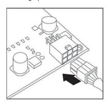
**Caution**: Make sure that all connectors are securely connected. Incorrect connections could prevent your computer from starting and could damage some components.
